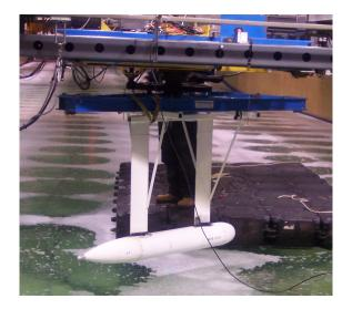
Fig. 6. A Phoenix AUV model (bare hull) suspended from the NRC-IOT Planar Motion Mechanism in the towing tank
