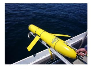
Fig. 2. Launching a glider over the side of a small fishing vessel
