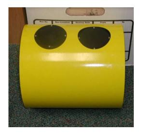
Fig. 15. Glider payload module for four puck-size sensors
