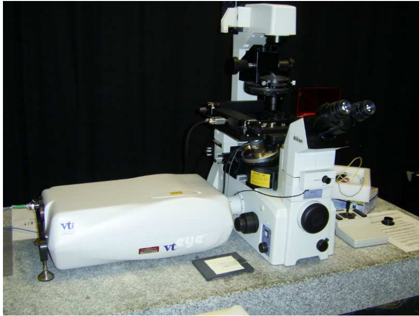
Figure 3.2: Nikon Eclipse TE2000-U with Visitech VT-Eye confocal.
