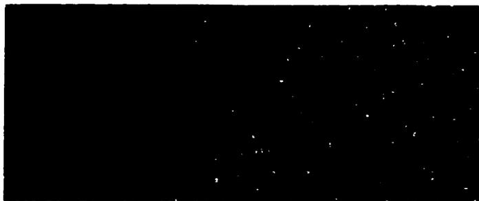
Figure 5.1: A “difference” image showing the NA interface. The images  $I_1$  and  $I_2$  in the difference image are separated by a time interval of 1 sec. to ensure that they are statistically independent. Shown is a  $450 \times 200$  pixel area of the image, corresponding to an area of  $\approx 0.6 \times 0.25$ mm area in a sample of 8CB. The lateral gradient  $dT/dx \approx 1^\circ\text{C}/\text{mm}$ .
