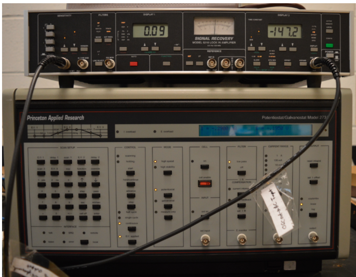
Figure 3.3: A potentiostat/galvanostat (Princeton Applied Research model 273A) attached to a lock-in amplifier (Signal Recovery model 5210) was used as an impedance spectrometer.
