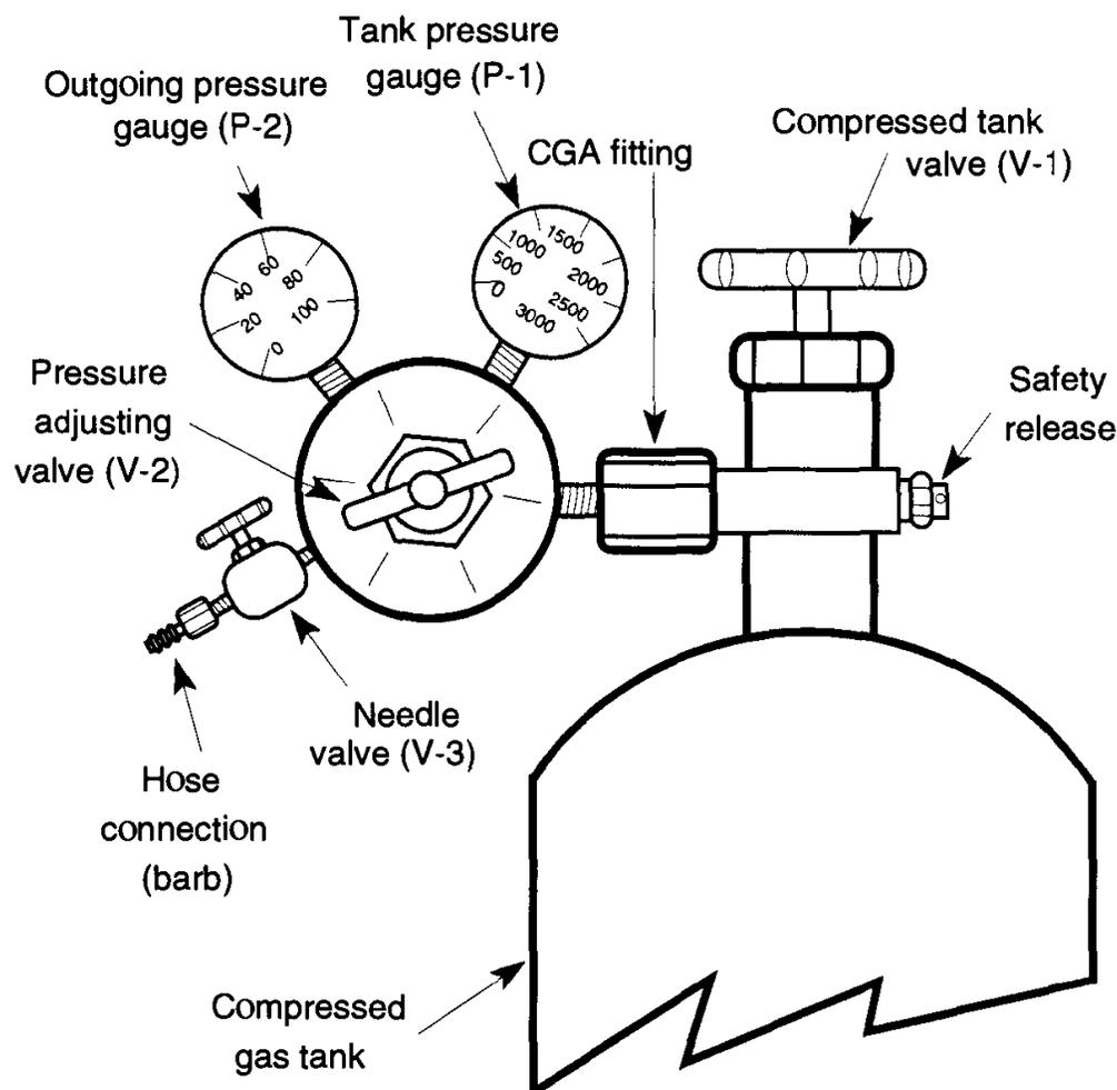
Fig. 5.4 Parts of the regulator.
