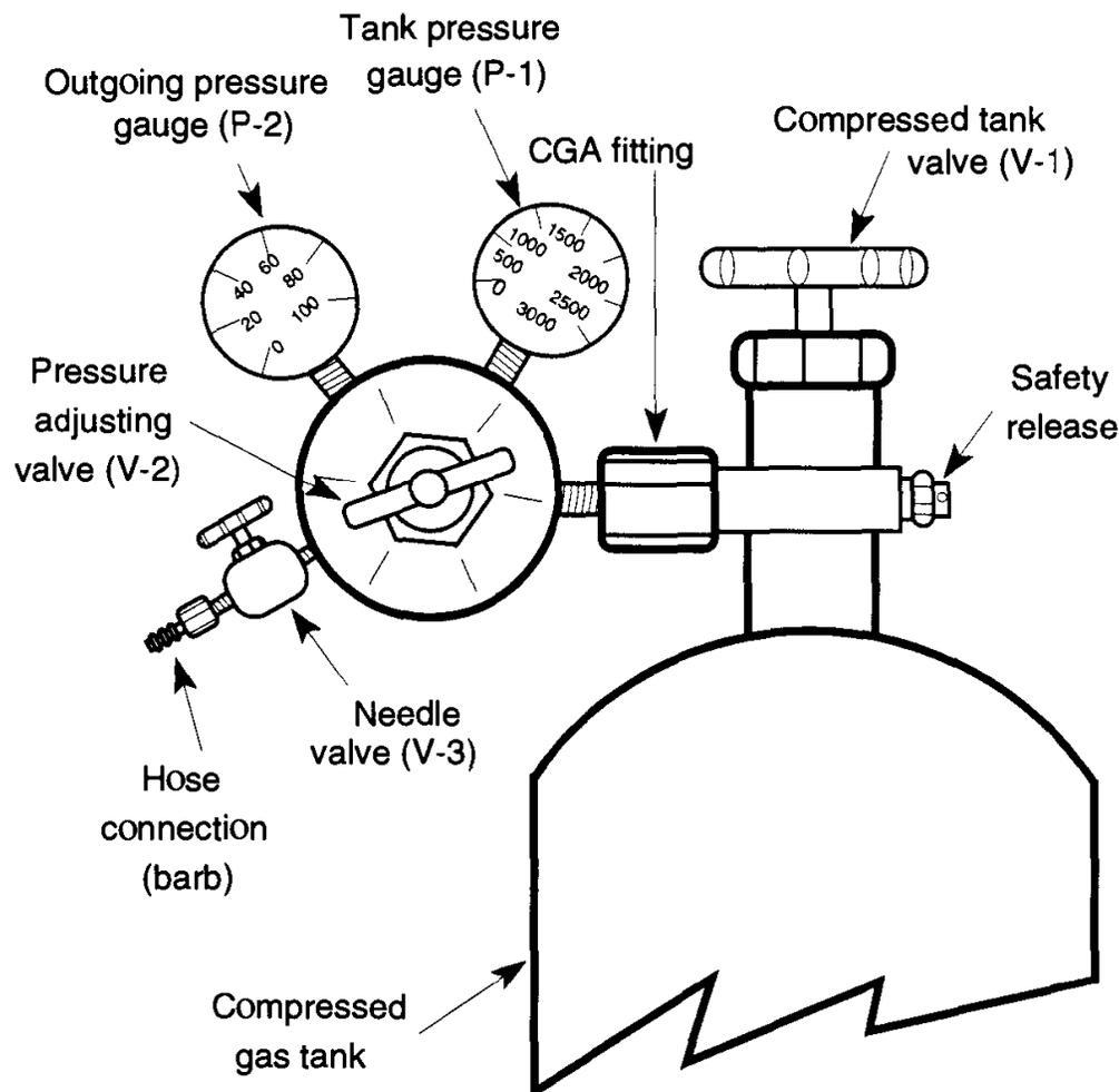
Fig. 5.4 Parts of the regulator.
