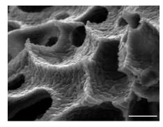
Ice templates. (Left) Nacre-like layers after removal of ice dendrites from solidification of alumina suspension in water. [Adapted from (12)] (Center) Starburst voids after removal of naphthalene dendrites from solidification of alumina sus-
