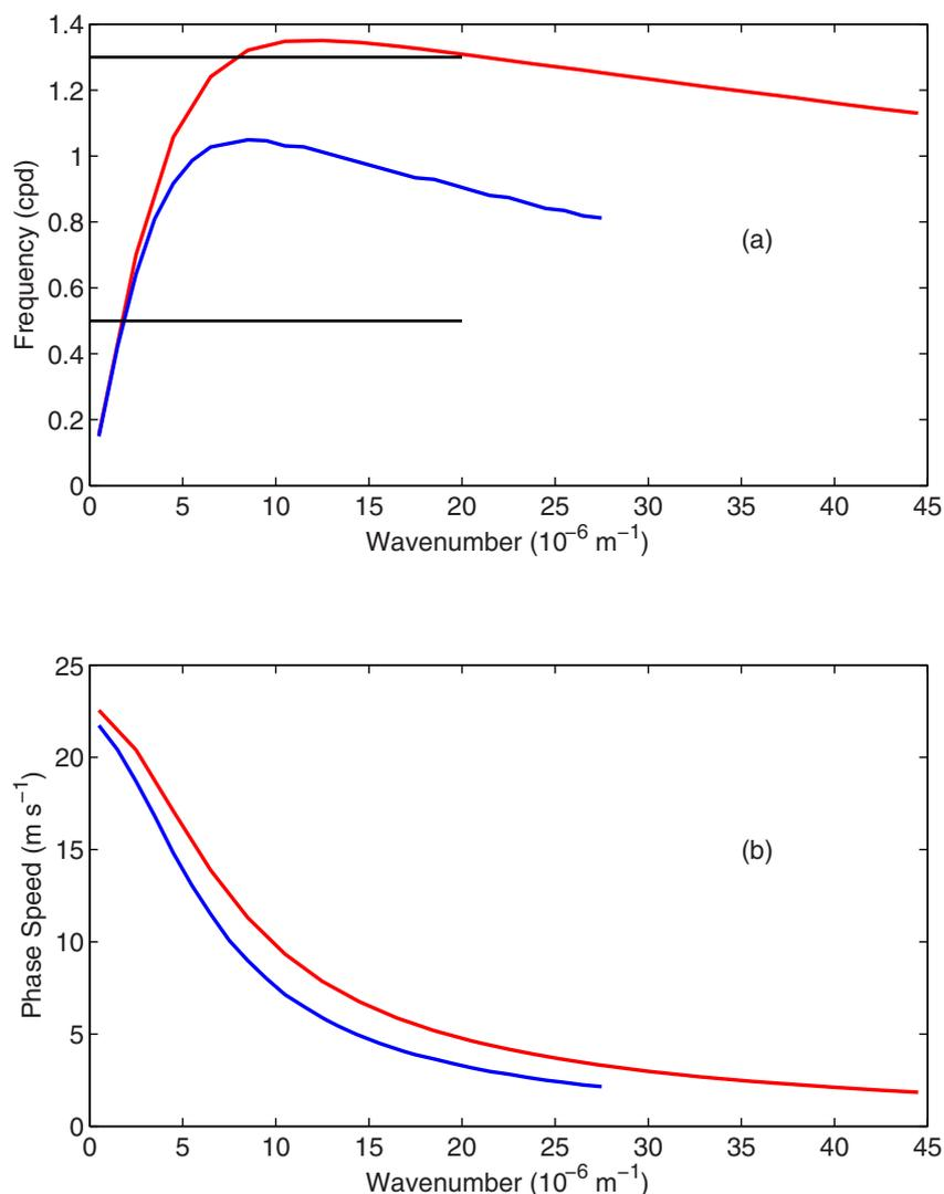
**Figure 6** | (a) Dispersion relationships for first-mode continental shelf waves and (b) phase speed as a function of the wavenumber at two transects near St. John's (blue curve) and Argientia (red curve) (See Fig. 1 for location). The two horizontal lines in (a) indicate the dominant frequencies of 0.5 and 1.3 cpd at St. John's and near Argientia, respectively.
