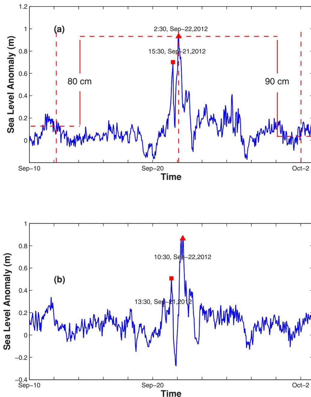
**Figure 3** | (a) Residual tide-gauge sea level anomalies at St. John's, and (b) Same as (a) but at Argentina. The vertical dashed lines indicate the times of the satellite passing before, during, and after Hurricane Igor. The solid triangles (squares) indicate the maximum surges (initial peaks) at St. John's and Argentina.
