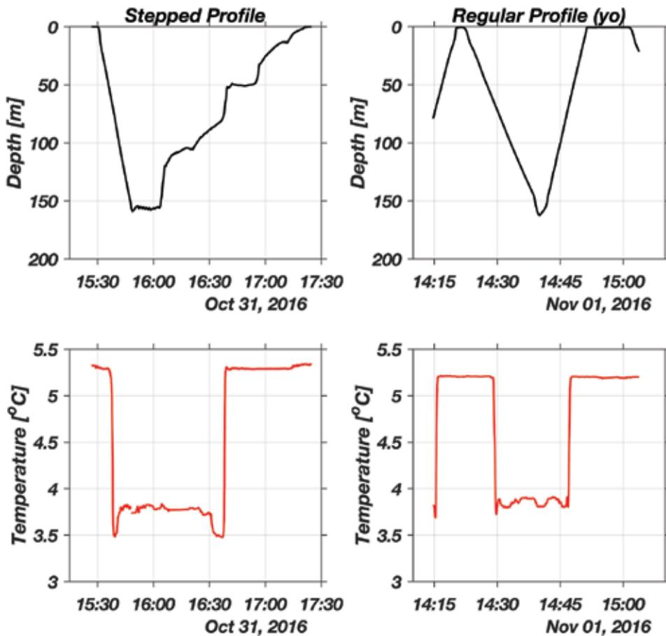
Figure 3: Comparison of yo and stepped profiles during the repeat sampling within section B.
