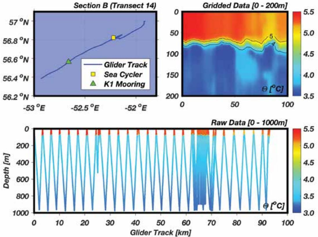
Figure 6: Typical transect in section B between K1 and SeaCycler. Note extra loop flown around SeaCycler mooring and increased data density at the mooring.
