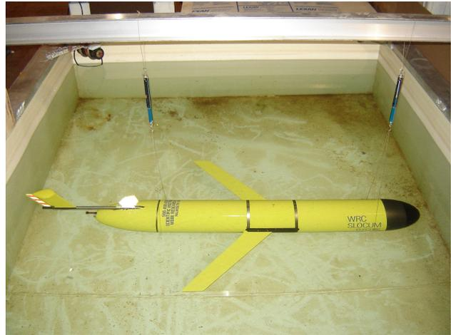
**Figure 3: Photograph of a SLOCUM glider suspended from two spring-scales being ballasted for zero pitch and zero roll angle in our freshwater ballast tank.**
