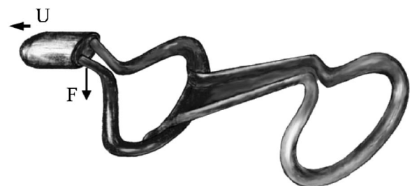
FIG. 4. Sketch of the vortex tubes behind a body applying the lift force periodically.
