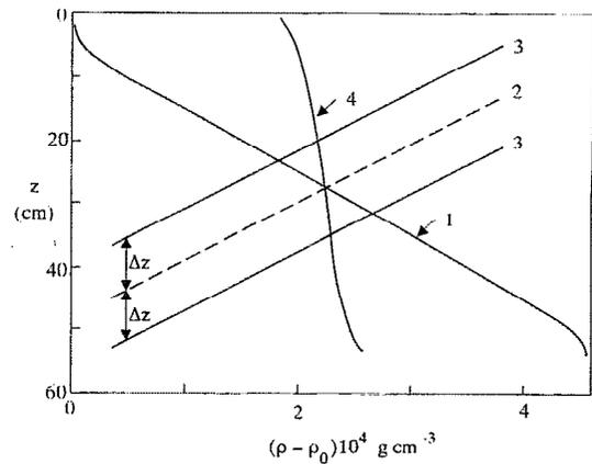
FIG. 5. Typical vertical density profiles measured before the overturning of the tank (1) and at the end of the experiment (4). The profiles after overturning in the vertical midplane of the tank (2) and at the front and back face walls (3) are also shown schematically.
