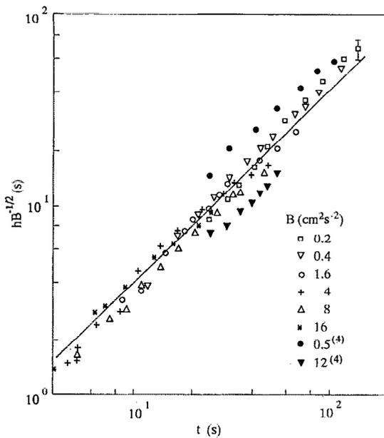
FIG. 2. Plot of the normalized width  $h/B^{1/2}$  of the convective region versus the time  $t$  measured from the beginning of the experiment. The data obtained in Ref. 4 are shown by (●) and (▼).
