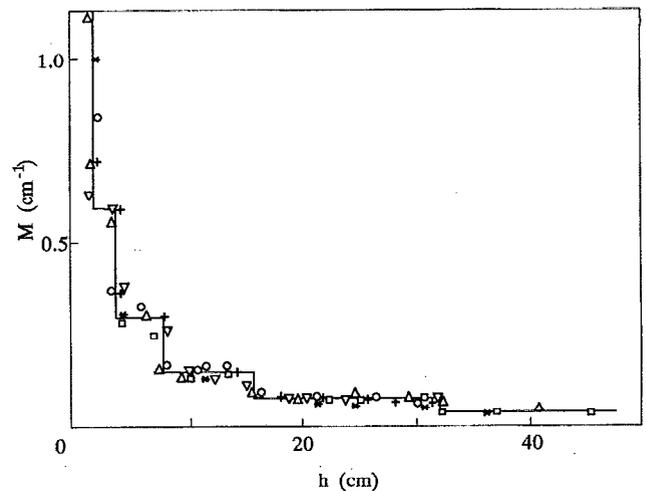
FIG. 3. Plot of the number  $M$  of convective elements per unit length versus the depth  $h$  of the convective region. The steplike solid line represents the theoretical prediction.
