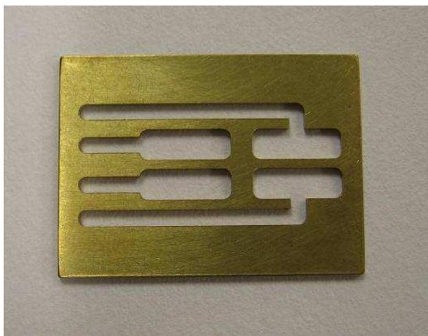
Figure 2.21: Brass mask for rotating field.
