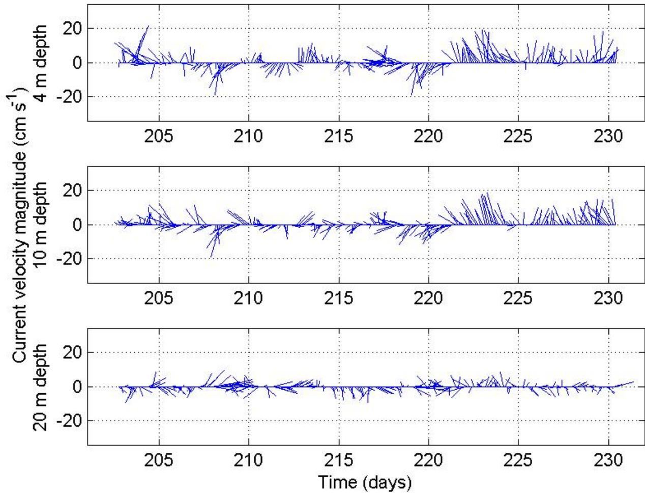
**Figure 2:** Magnitude and direction for a) wind stress and b) current velocity at surface (4 m), middle (10 m) and bottom (20 m) depths for mooring M2. Vectors shown represent averaged values of each 3 hour segment of the entire sampling period.
