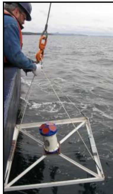
Figure 9 Deployment of the ADCP mooring
