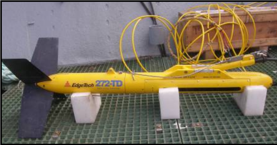
Figure 7, The Edge Tech 272-TD sidescan sonar
