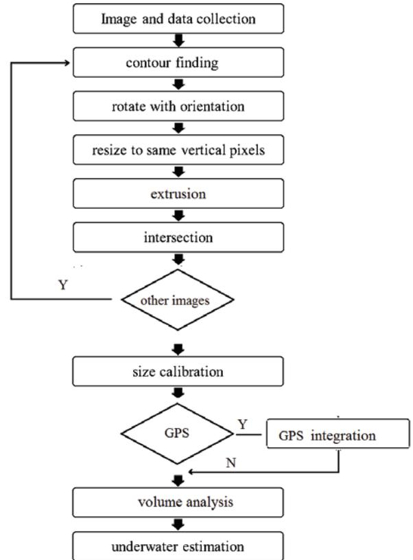
Fig. 7 Flow chart of 3-D Modelling of Above-water Iceberg
