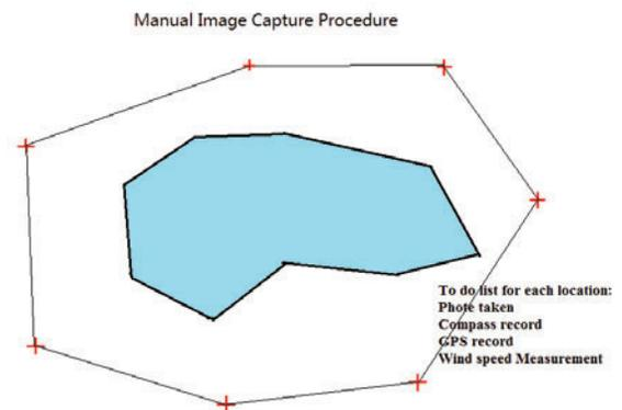
Fig. 4 Arbitrary waypoints for data collection, and the “to-do list” for each location.
