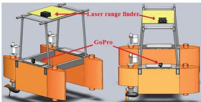
Fig. 3 The placement of GoPro and Laser range finder on ASC.
