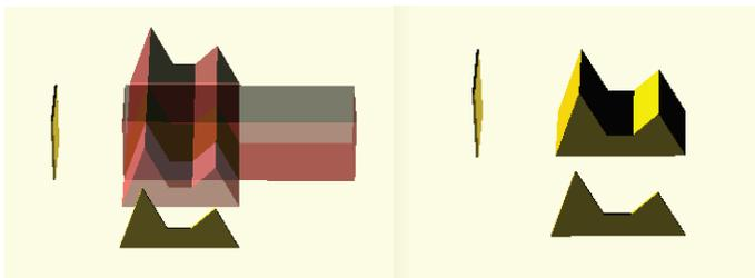
Fig 1. Simplified volume intersection algorithm. The left image is the extrusion of two different silhouettes (the front view is an irregular shape, and the left view is a square). The right image shows the isometric view of the object after intersection.
