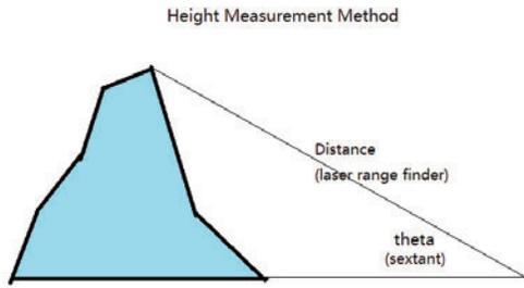
Fig. 5 Height measurement method. For size calibration, we need to measure the height of the iceberg using triangulation with range and elevation angle.
