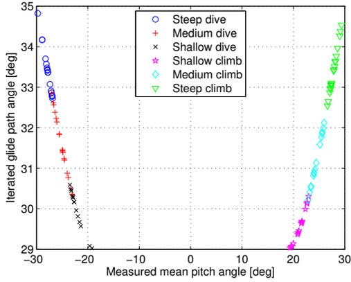
Fig. 11. Glide path angle vs glider pitch angle
