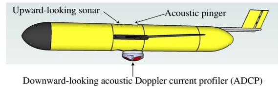
Fig. 16. A glider equipped with an ADCP
