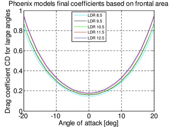
Fig. 8. Drag coefficient CD for the five models
