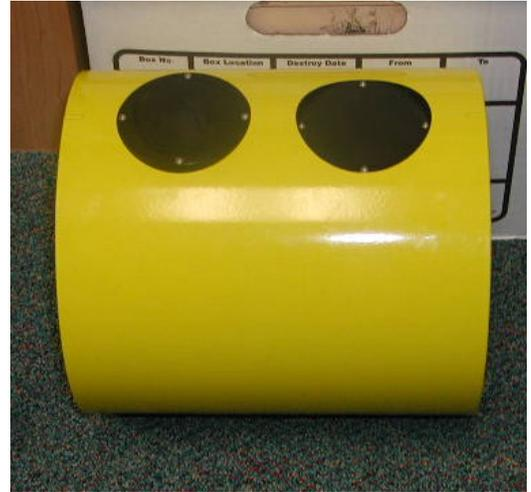
Fig. 15. Glider payload module for four puck-size sensors
