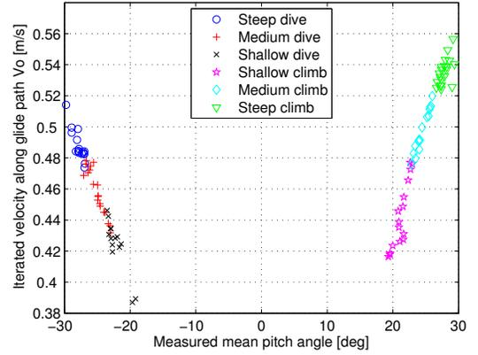
Fig. 12. Glide speed vs glider pitch angle
