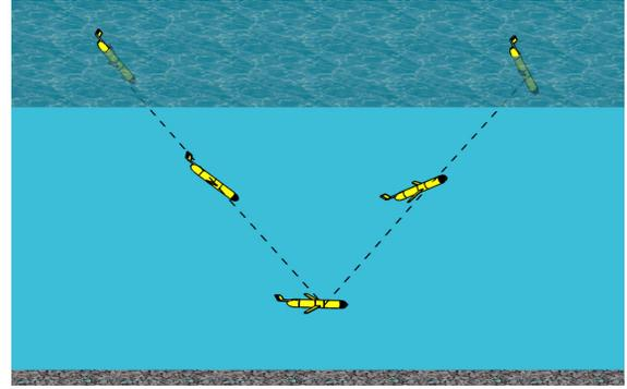
Fig. 1. Example saw-tooth pattern for gliding
