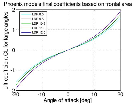
Fig. 9. Lift coefficient CL for the five models
