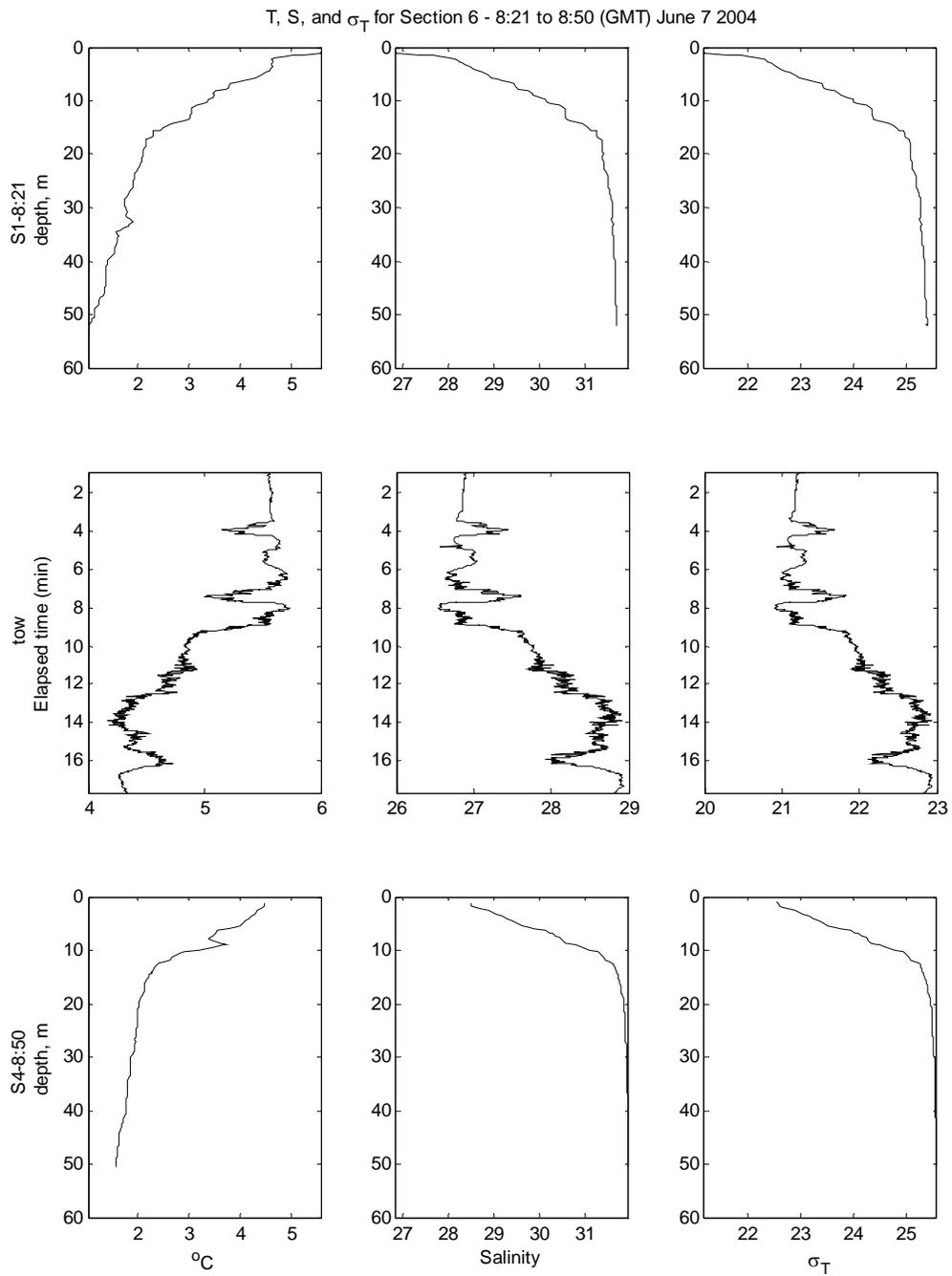
**Figure 41: Vertical and horizontal temperature, Salinity and sigma-t profiles from S1 to S4, 8:21 to 8:50 GMT June 7 2004.**
