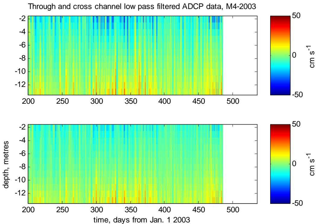
**Figure 25: ADCP data for M4-2003 rotated for through and cross channel flow at each depth bin according to the angles specified in Fig. 16**
