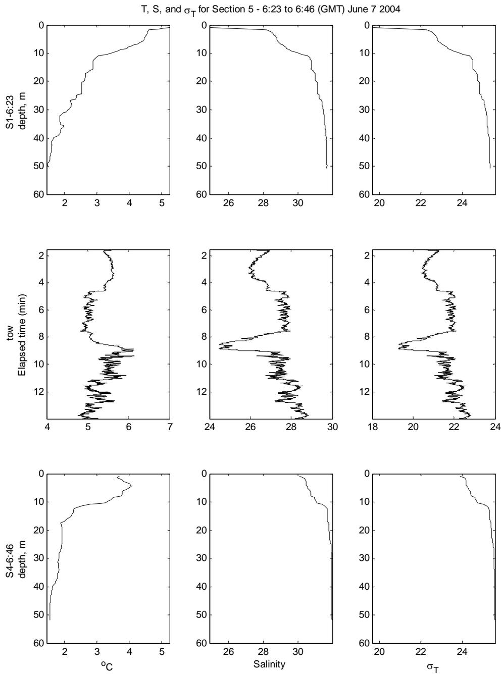
**Figure 40: Vertical and horizontal temperature, Salinity and sigma-t profiles from S1 to S4, 6:23 to 6:45 GMT June 7 2004.**
