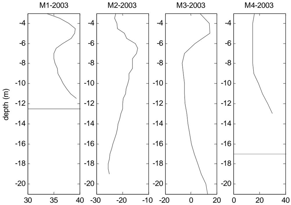
**Figure 16: Major axis angles for 2003 data at each depth bin calculated using Emery, 1997 pp 325. Angles are given in degrees, where  $0^\circ$  is East. The horizontal line indicates the bottom.**
