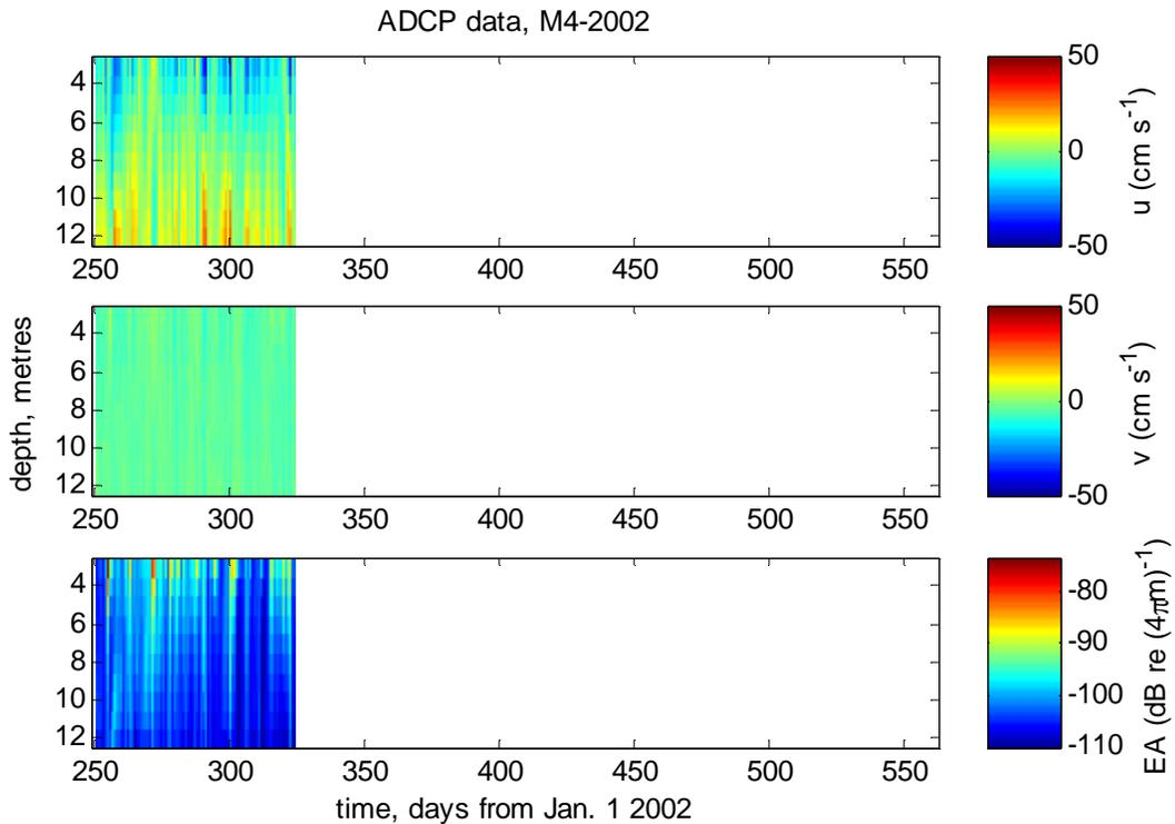
**Figure 8: Low pass filtered ADCP data from mooring M4-2002. Cutoff is 30 hours. Top: East-west speed (cm/s). Middle: North-south speed (cm/s). Bottom: Spherically corrected backscatter intensity.**
