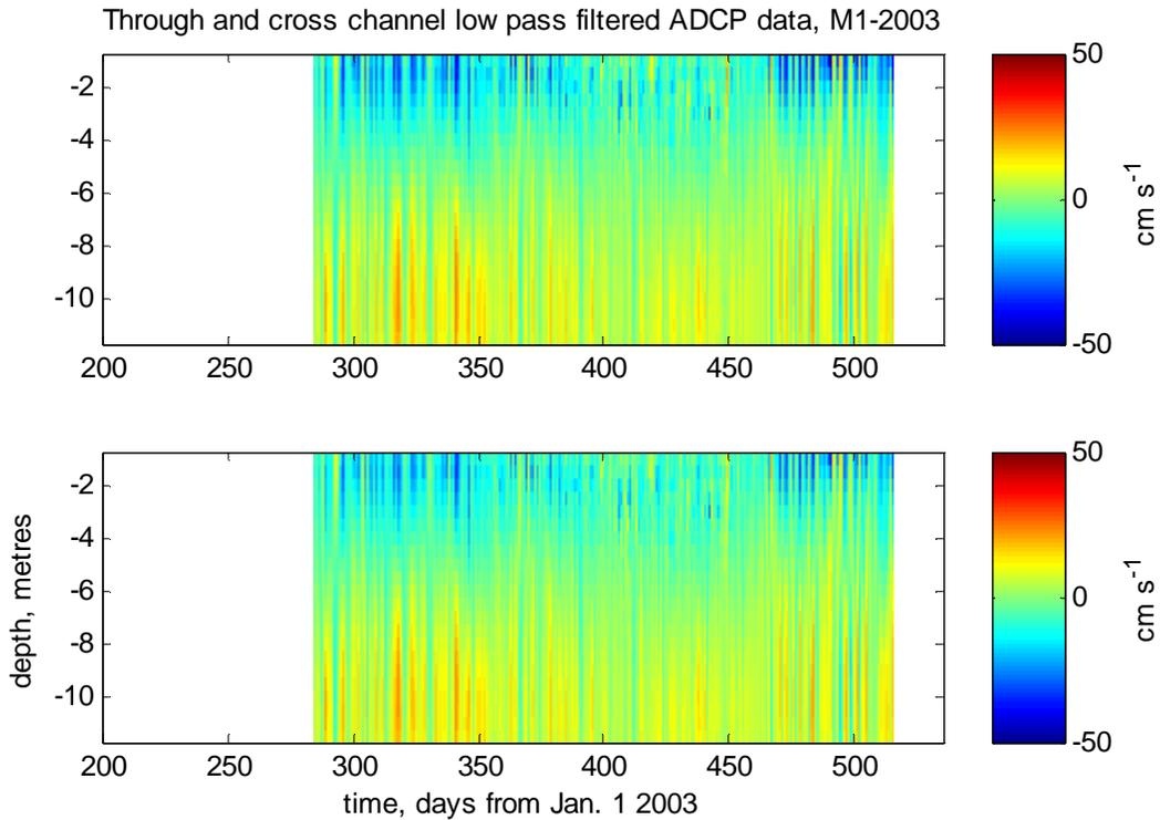
**Figure 22: ADCP data for M1-2003 rotated for through and cross channel flow at each depth bin according to the angles specified in Fig. 16**
