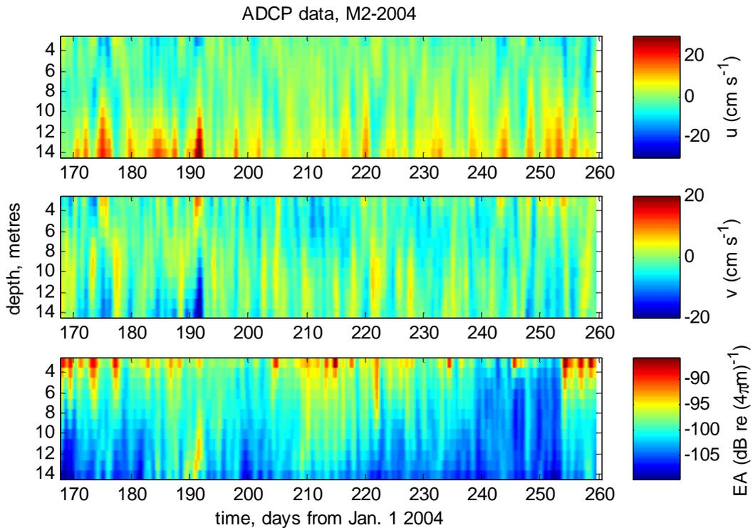
**Figure 14: Low pass filtered ADCP data from mooring M2-2004. Cutoff is 30 hours. Top: East-west speed (cm/s). Middle: North-south speed (cm/s). Bottom: Spherically corrected backscatter intensity.**
