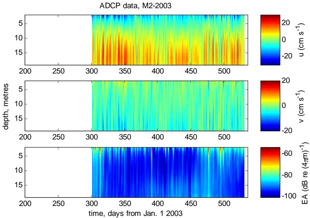
**Figure 10: Low pass filtered ADCP data from mooring M2-2003. Cutoff is 30 hours. Top: East-west speed (cm/s). Middle: North-south speed (cm/s). Bottom: Spherically corrected backscatter intensity**
