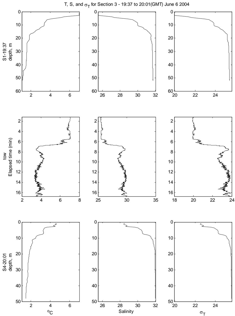
**Figure 38: Vertical and horizontal temperature, Salinity and sigma-t profiles from S1 to S4, 19:37 to 20:01 GMT June 6 2004.**
