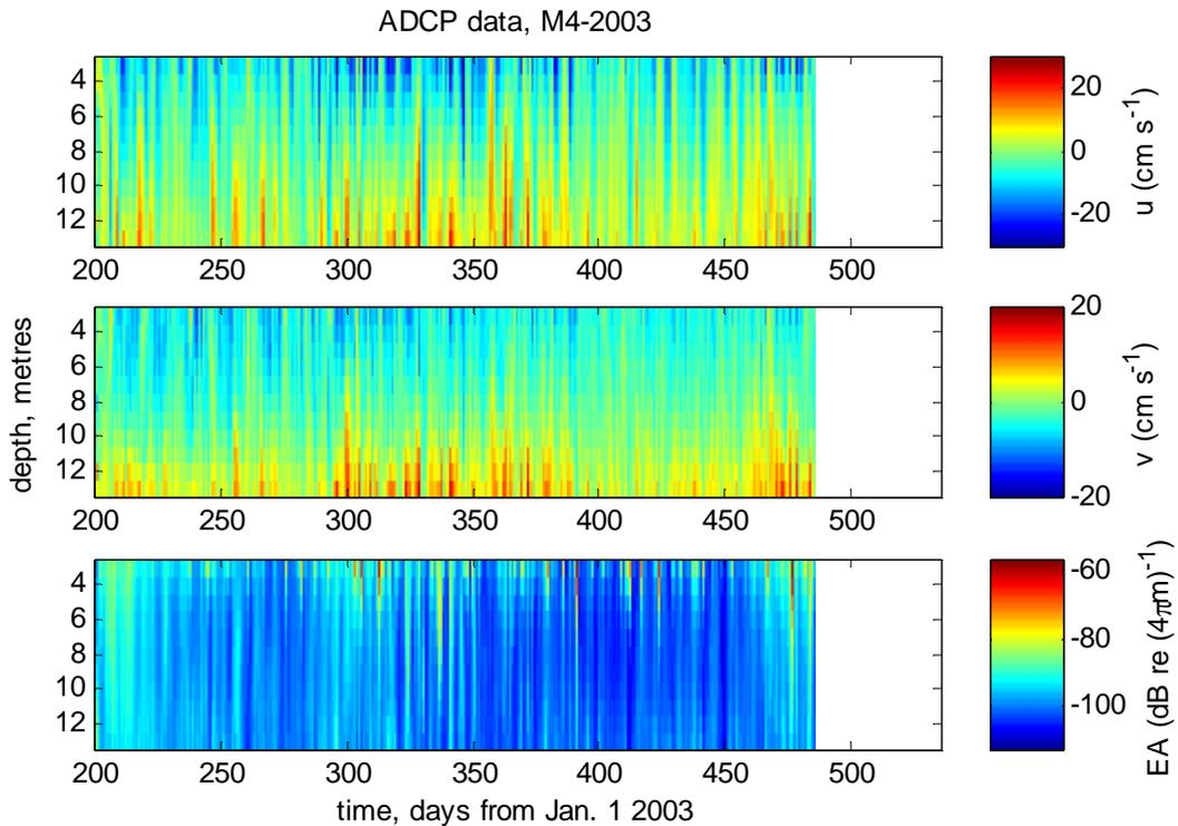
**Figure 12: Low pass filtered ADCP data from mooring M4-2003. Cutoff is 30 hours. Top: East-west speed (cm/s). Middle: North-south speed (cm/s). Bottom: Spherically corrected backscatter intensity.**
