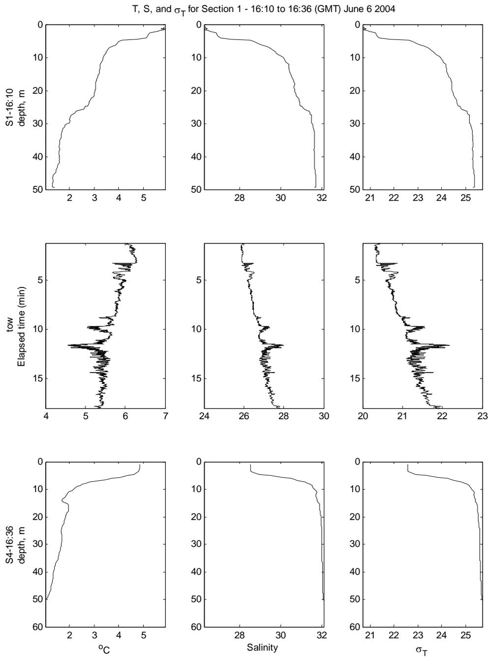
**Figure 36: Vertical and horizontal temperature, salinity and sigma-t profiles from S1 to S4, 16:10 to 16:36 GMT June 6 2004.**
