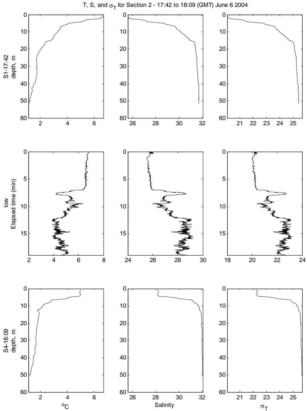
**Figure 37: Vertical and horizontal temperature, Salinity and sigma-t profiles from S1 to S4, 17:42 to 18:09 GMT June 6 2004.**
