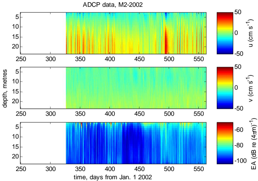
**Figure 6: Low pass filtered ADCP data from mooring M2-2002. Cutoff is 30 hours. Top: East-west speed (cm/s). Middle: North-south speed (cm/s). Bottom: Spherically corrected backscatter intensity.**
