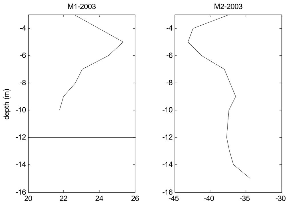
**Figure 17: Major axis angles for 2002 data at each depth bin calculated using Emery, 1997 pp 325. Angles are given in degrees, where  $0^\circ$  is East. The horizontal line indicates the bottom.**
