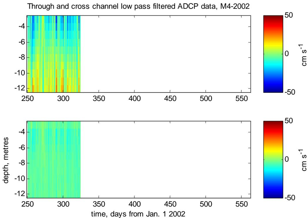
**Figure 21: ADCP data for M4-2002 rotated for through and cross channel flow at each depth bin according to the angles specified in Fig. 15**
