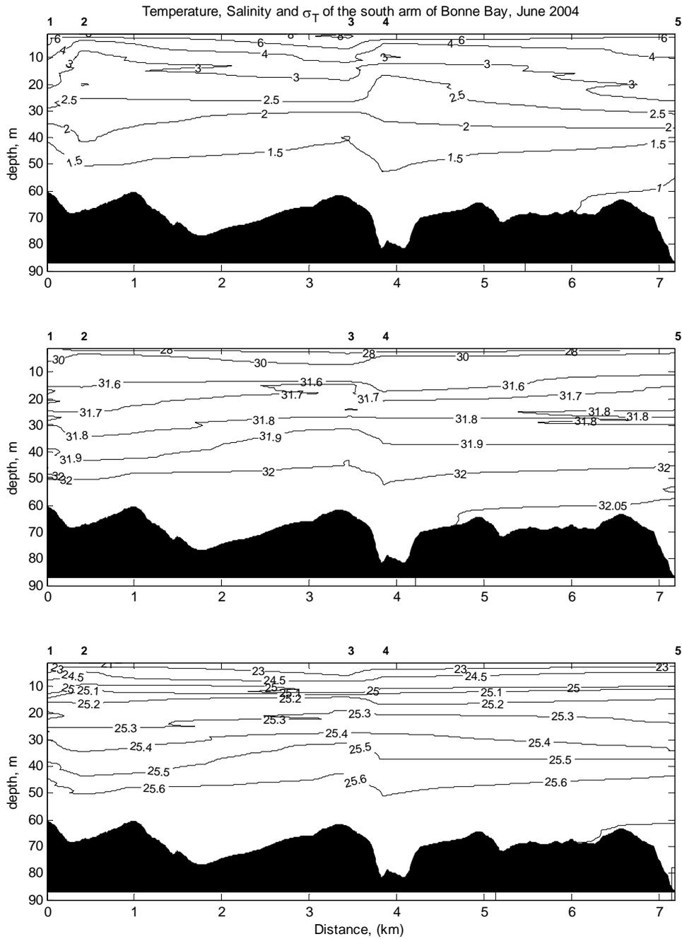
**Figure 44: Temperature, salinity and sigma-t along the South arm of Bonne Bay, June 2004. Numbers indicate CTD stations in Fig. 43. Stations 2 and 4 were collected June 9 2004, while stations 1, 3 and 5 were collected June 13 2004. This is the cause of the ‘bumpiness’ of the contours near the stations.**
