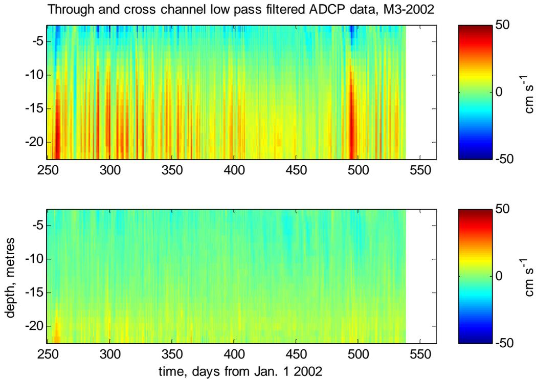
**Figure 20: ADCP data for M3-2002 rotated for through and cross channel flow at each depth bin according to the angles specified in Fig. 15**
