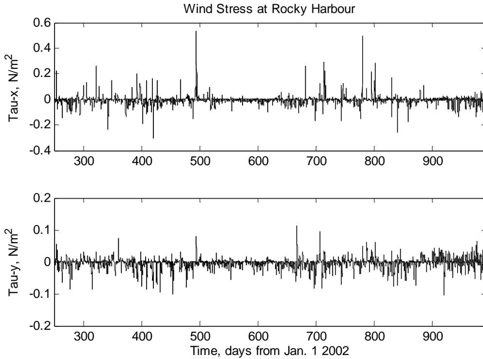
**Figure 28: Wind stress at Rocky Harbour over the period for which there is ADCP data. Calculated according to Gill 1982.**
