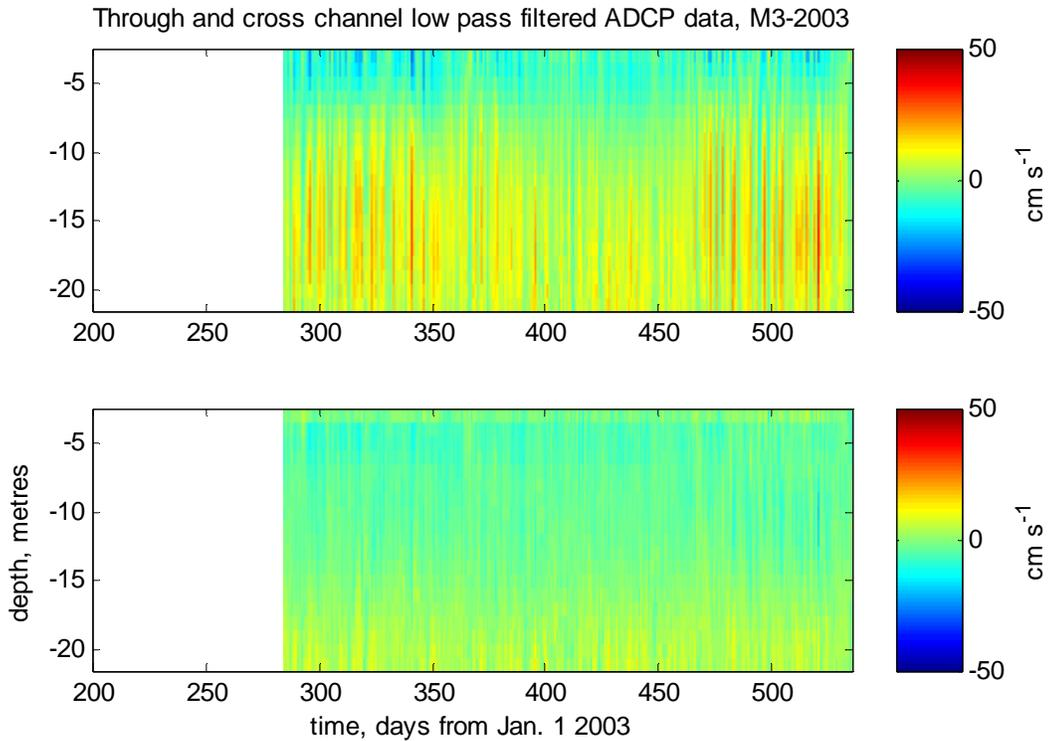
**Figure 24: ADCP data for M3-2003 rotated for through and cross channel flow at each depth bin according to the angles specified in Fig. 16**
