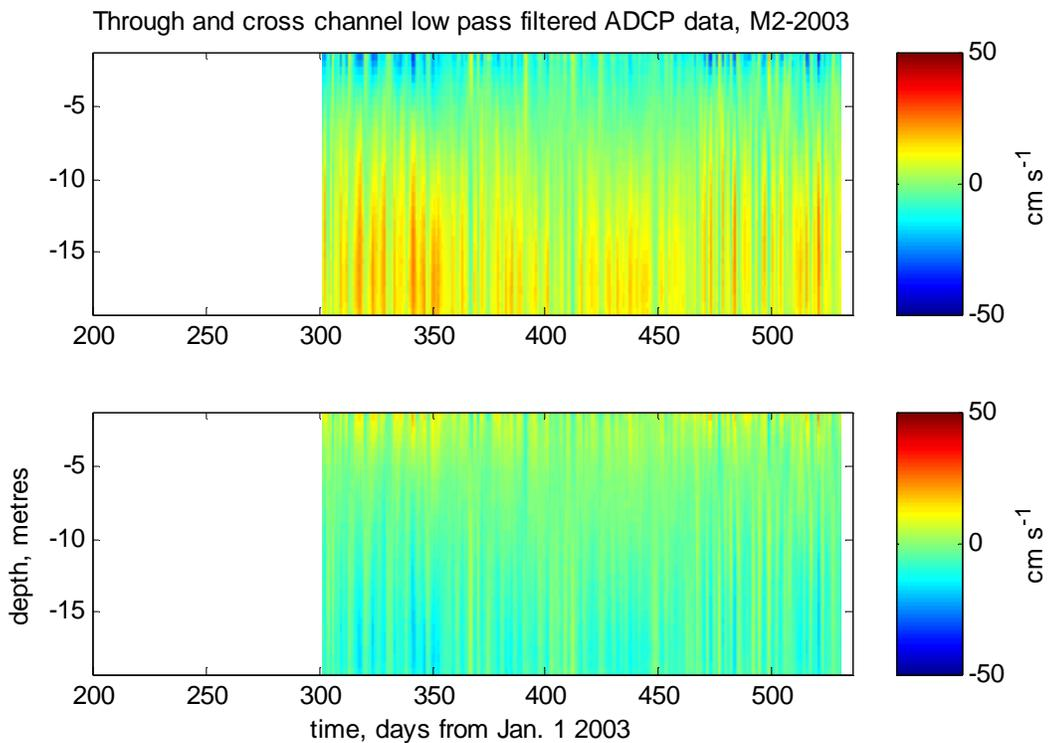
**Figure 23: ADCP data for M2-2003 rotated for through and cross channel flow at each depth bin according to the angles specified in Fig. 16**
