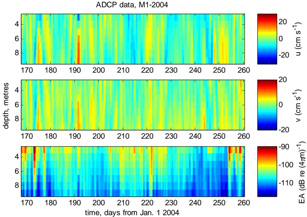
**Figure 13: Low pass filtered ADCP data from mooring M1-2004. Cutoff is 30 hours. Top: East-west speed (cm/s). Middle: North-south speed (cm/s). Bottom: Spherically corrected backscatter intensity.**
