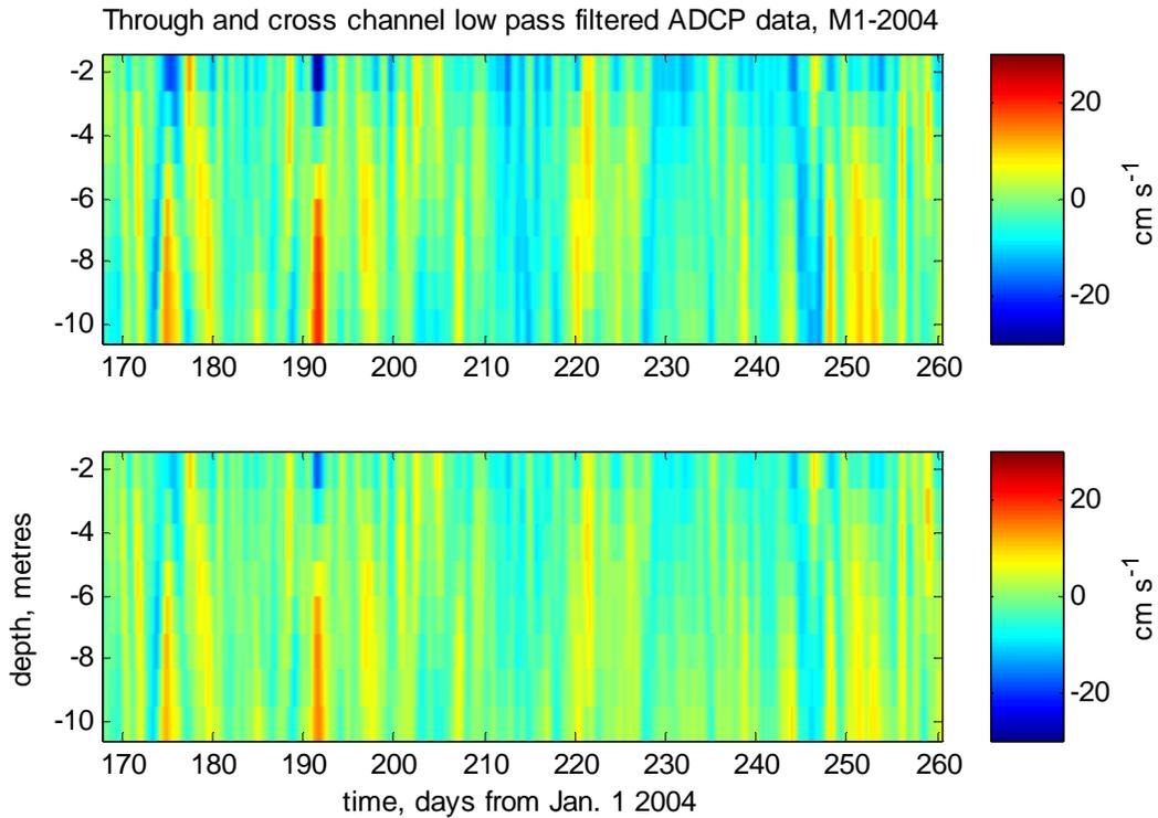
**Figure 26: ADCP data for M1-2004 rotated for through and cross channel flow at each depth bin according to the angles specified in Fig. 17**
