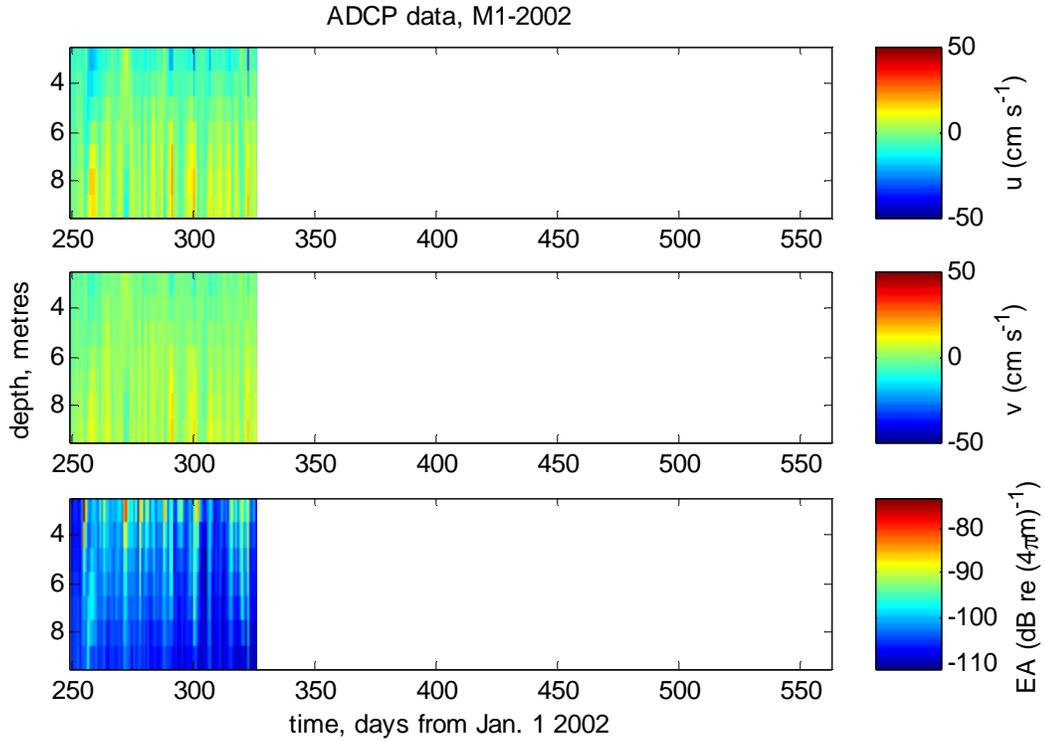
**Figure 5: Low pass filtered ADCP data from mooring M1-2002. Cutoff is 30 hours. Top: East-west speed (cm/s). Middle: North-south speed (cm/s). Bottom: Spherically corrected backscatter intensity.**
