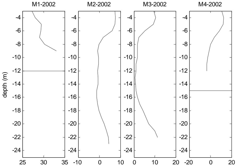
**Figure 15: Major axis angles for 2002 data at each depth bin calculated using Emery, 1997 pp 325. Angles are given in degrees, where  $0^\circ$  is East. The horizontal line indicates the bottom.**
