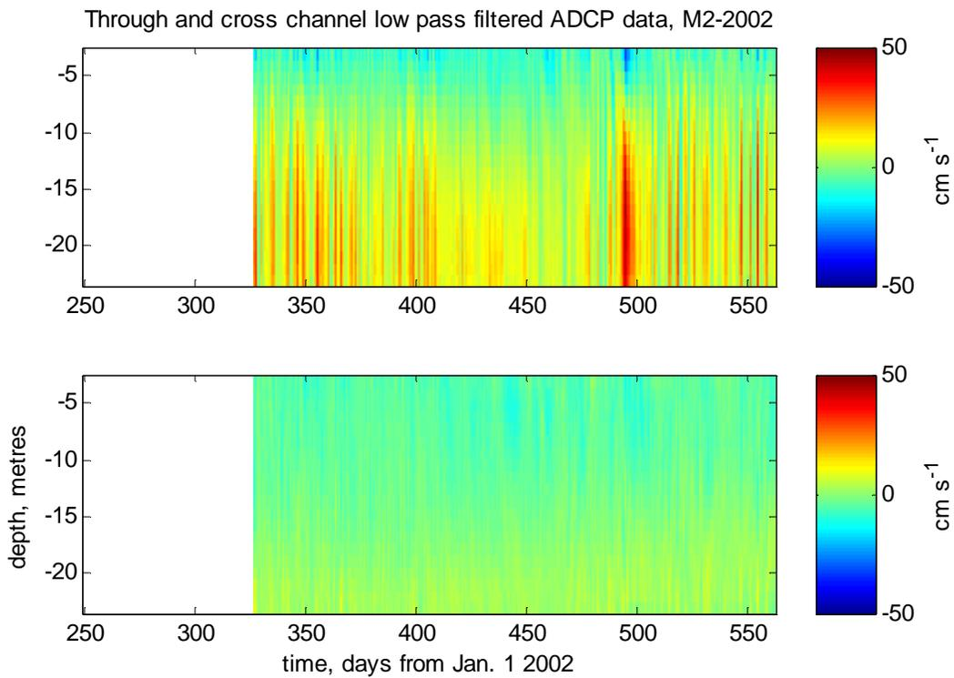
**Figure 19: ADCP data for M2-2002 rotated for through and cross channel flow at each depth bin according to the angles specified in Fig. 15**
