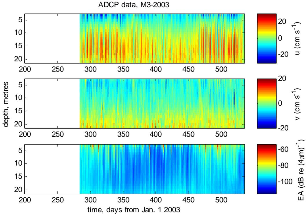
**Figure 11: Low pass filtered ADCP data from mooring M3-2003. Cutoff is 30 hours. Top: East-west speed (cm/s). Middle: North-south speed (cm/s). Bottom: Spherically corrected backscatter intensity.**
