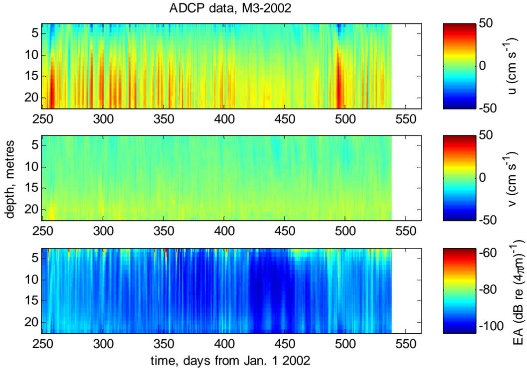
**Figure 7: Low pass filtered ADCP data from mooring M3-2002. Cutoff is 30 hours. Top: East-west speed (cm/s). Middle: North-south speed (cm/s). Bottom: Spherically corrected backscatter intensity.**
