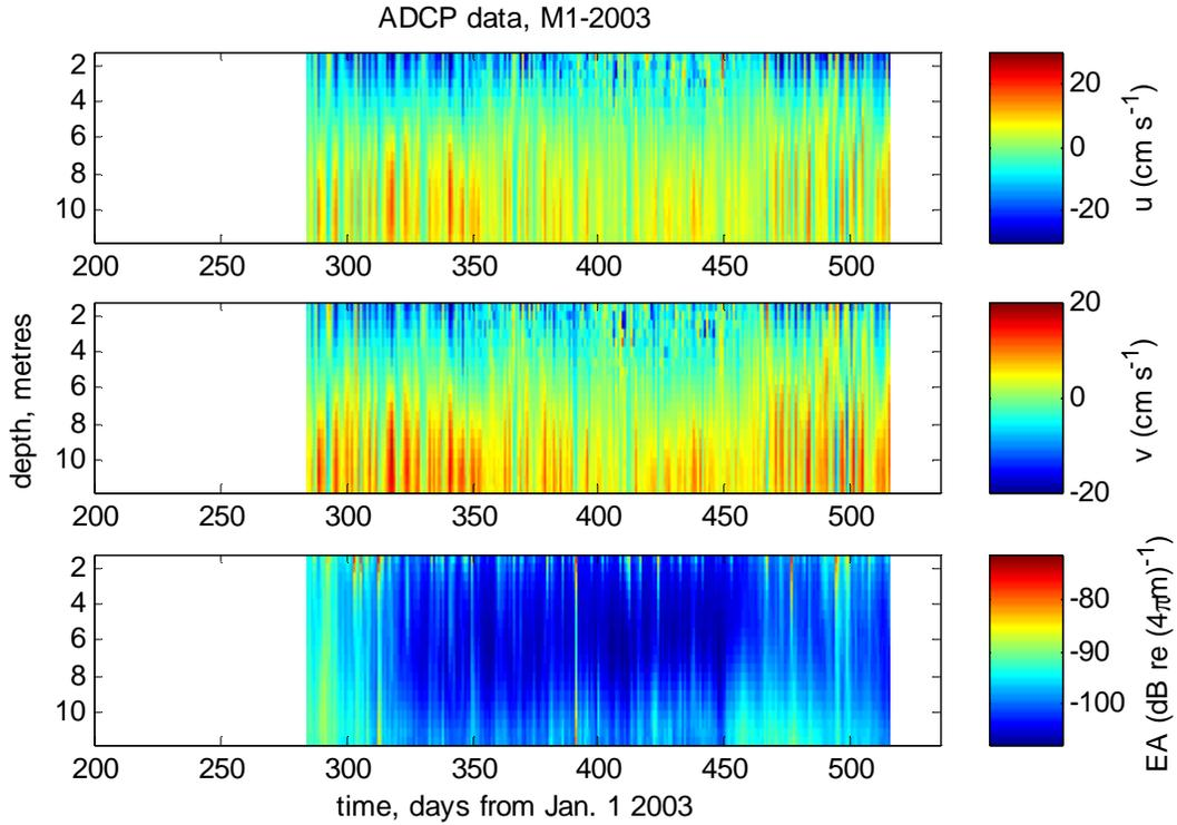
**Figure 9: Low pass filtered ADCP data from mooring M1-2003. Cutoff is 30 hours. Top: East-west speed (cm/s). Middle: North-south speed (cm/s). Bottom: Spherically corrected backscatter intensity.**
