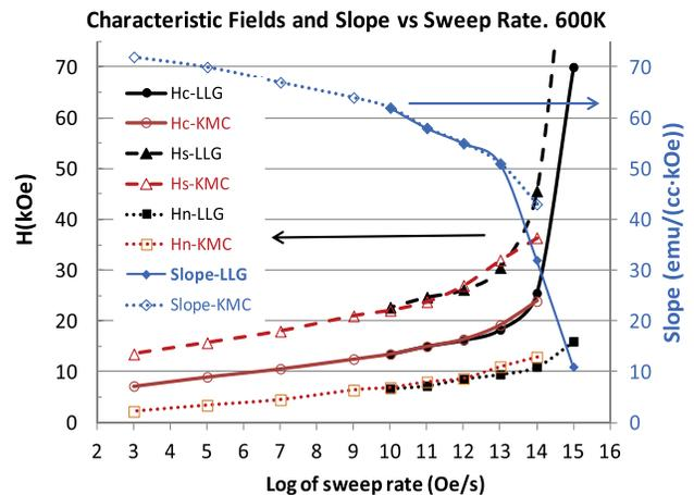
FIG. 2. Comparison of coercivity ( $H_c$ ), saturation ( $H_s$ ), and nucleation ( $H_n$ ) field values as well as slopes near  $H_c$ , estimated from Fig. 1.
