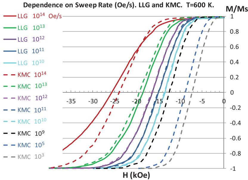
FIG. 1. Comparison of KMC and LLG results for *MH* loops at  $T = 600$  K at various sweep rates  $R$  (in Oe/s).
