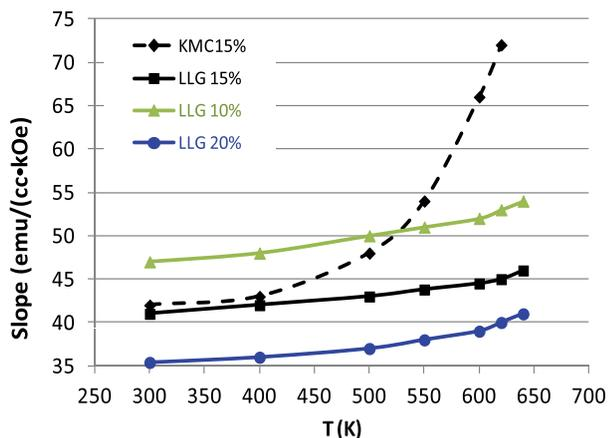
FIG. 5. Slope vs temperature for slow (KMC) and fast (LLG) sweep rates. Also shown is the effect of varying the distribution sigmas on  $M_s$  and  $K$  for the LLG simulations.
