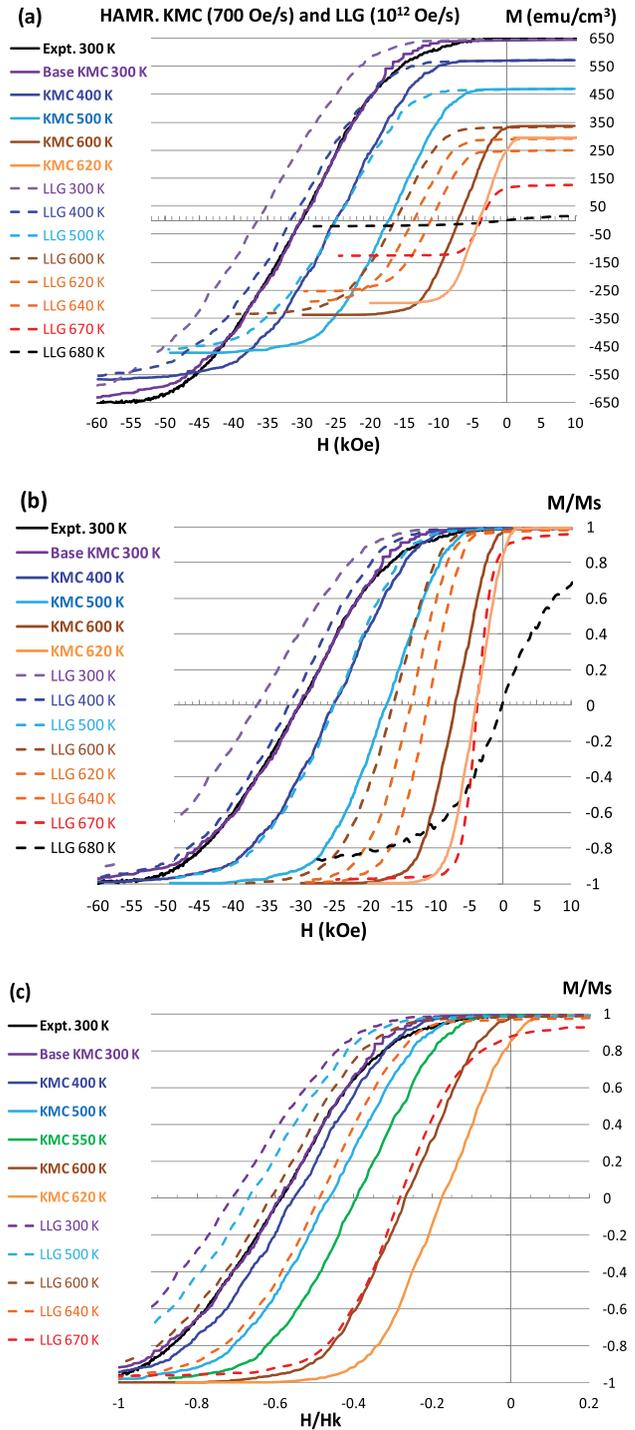
FIG. 3. Three representations of the same simulation results for  $MH$  loops at slow and fast sweep rates with increasing temperature: (a)  $M$  vs  $H$ , (b)  $M/M_s$  vs  $H$ , and (c)  $M/M_s$  vs  $H/H_K$ . Fewer loops are shown in (c) for clarity. Note that the similarity between some loops at the different sweep rates for different values  $T$  is accidental.
