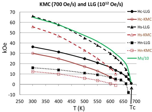
FIG. 4. Nucleation, coercivity, and saturation fields as a function of temperature estimated from Fig. 3. Also shown is  $M(T)$  used in the simulations taken from the 9 nm results of Ref. 12.
