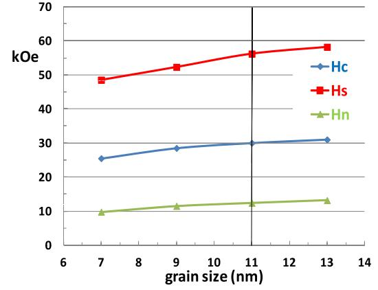
Fig. 6. Dependence of the coercivity  $H_c$ , saturation field  $H_s$ , and nucleation field  $H_n$  on grain size from the results in Fig. 2.
