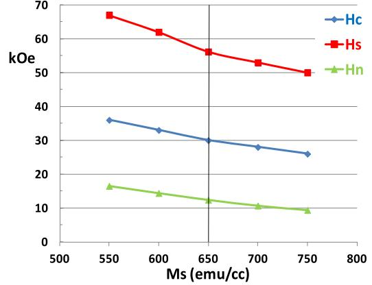
Fig. 7. Dependence of  $H_c$ ,  $H_s$ , and  $H_n$  on the saturation magnetization from the results in Fig. 3.
