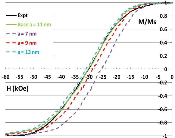
Fig. 2. Impact of lateral grain size dimension ( $a$ ) on  $M$ - $H$  loops.
