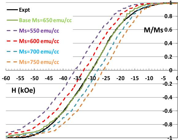
Fig. 3. Impact of variations in the saturation magnetization on  $M$ – $H$  loops.
