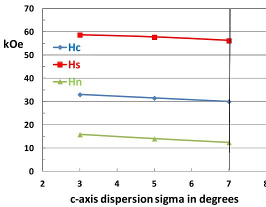
Fig. 9. Dependence of  $H_c$ ,  $H_s$ , and  $H_n$  on the anisotropy axis dispersion from the results in Fig. 5.
