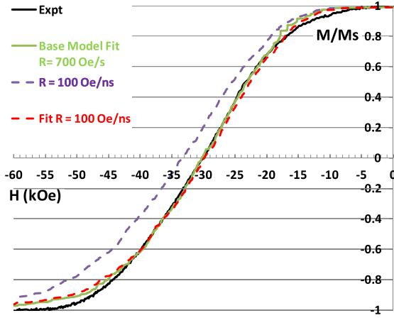
Fig. 1. Experimental HAMR media loop at 300 K and a sweep rate of  $R = 700$  Oe/s. Separate fitted simulations were performed at the experimental value of  $R$  as well as typical LLG rate of  $R = 100$  Oe/ns. Purple: result of using the slow sweep-rate (700 Oe/s) fitted parameters in a fast sweep rate (100 Oe/ns) simulation.
