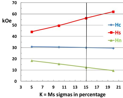
Fig. 8. Dependence of  $H_c$ ,  $H_s$ , and  $H_n$  on the standard deviation in anisotropy and magnetization from the results in Fig. 4.
