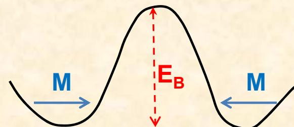
Surface spins are pinned into a state with the direction of  $M$  fixed.
