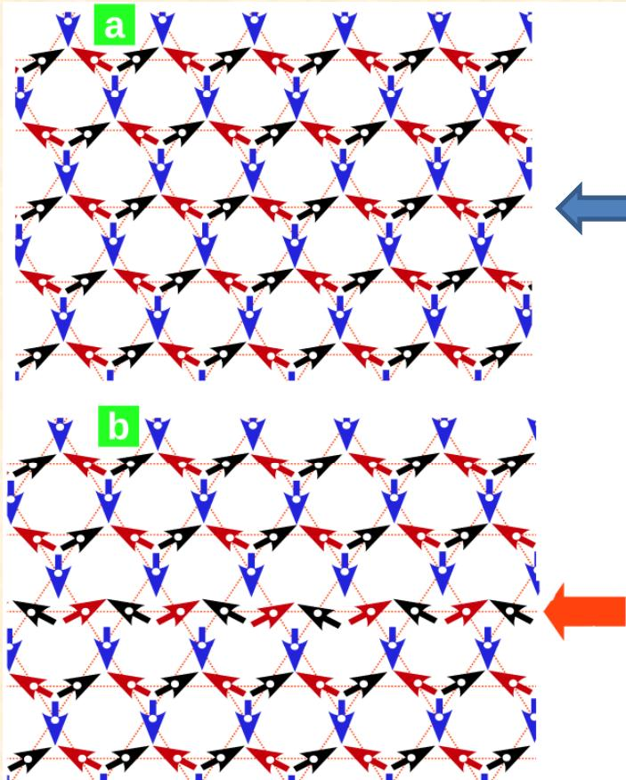
' $q=0$ ' magnetic structure  $\Rightarrow$  3 spins around each triangle at  $120^\circ$
