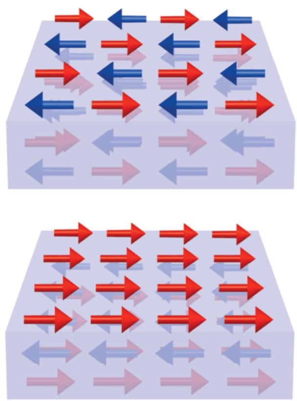
The atomic-scale *Roughness* can create uncompensated spins (red)
