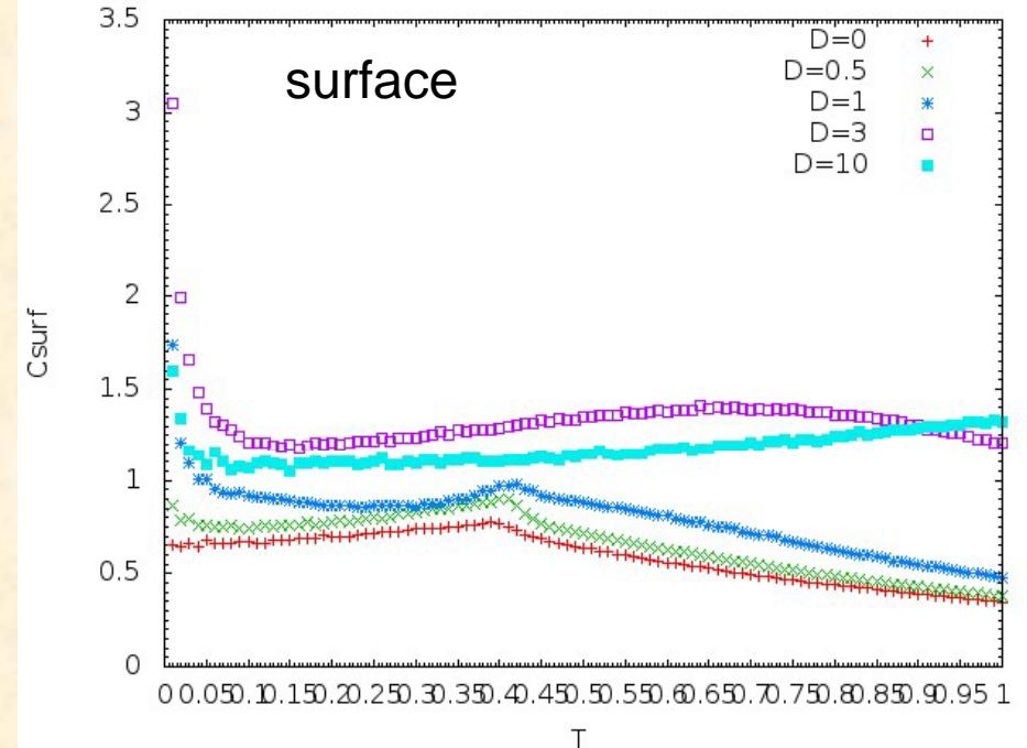
At large  $D$  surface spins do not show a sharp peak in specific heat
