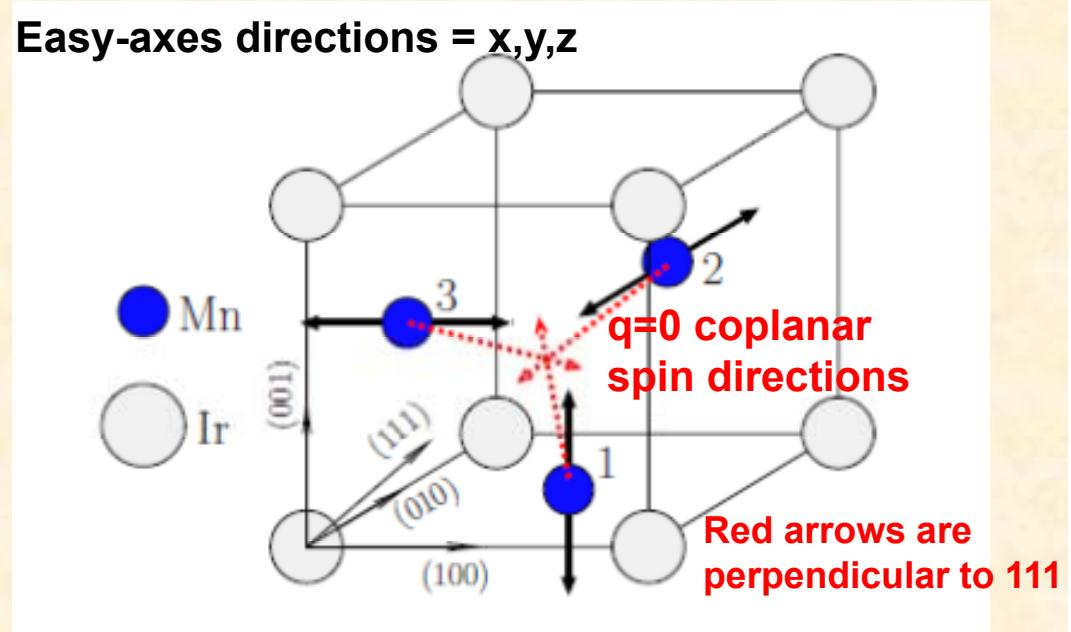
**Mn moments are *not* aligned in the easy-axes directions for the coplanar q=0 spin structure.**
