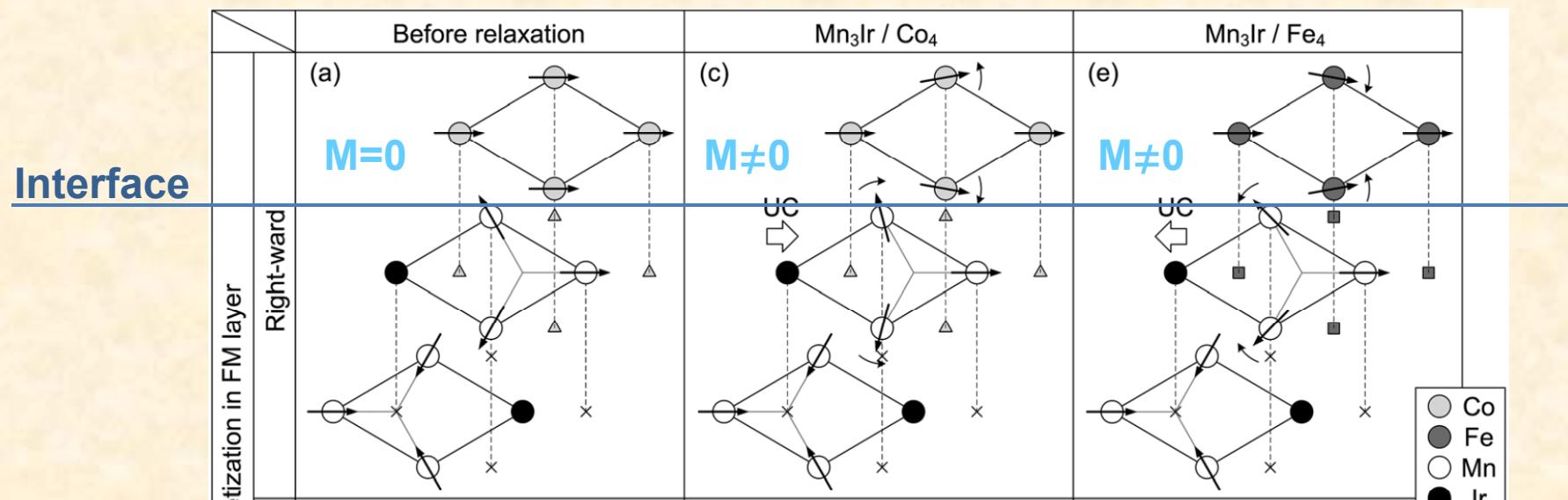
Interaction with ferromagnetic layer induces a net moment in surface Mn spins.
