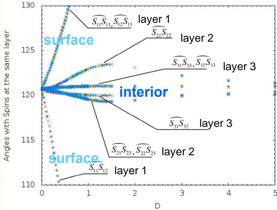
D causes **one** of the three spins in a surface triangle to point up (down), the other two mostly down (up).
