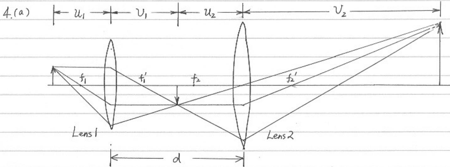
In order to design the system of two lenses with magnification of +30,
