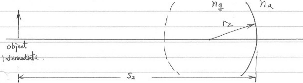
$$\frac{n_g}{s_2} + \frac{n_a}{s'_2} = \frac{n_a - n_g}{r_2}$$
