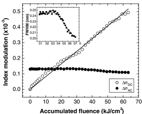
Fig. 3. DC and AC index modulations of the FBG as a function of accumulated femtosecond laser fluence. The inset is the change of the FWHM grating bandwidth. The single pulse fluence was  $124 \text{ mJ/cm}^2$ .
