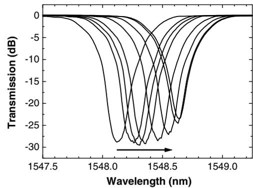
Fig. 1. Resonance wavelength shift in the transmission spectra of a FBG following uniform post laser exposure by a deep ultraviolet femtosecond laser at 258 nm. The spectra correspond to pristine FBG and the FBG after femtosecond laser exposure with accumulated fluences of 9.9, 19.8, 29.7, 39.6, 49.5, 59.4 and 63.3 kJ/cm<sup>2</sup> from left to right. The resonance wavelength shifts from initial 1548.12 to 1548.64 nm at 63.3 kJ/cm<sup>2</sup>.
