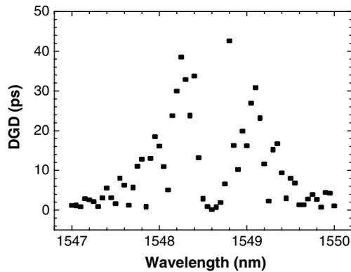
Fig. 4. Differential group delay (DGD) as a function of wavelength for the FBG after uniform femtosecond laser exposure with an accumulated fluence of  $63.3 \text{ kJ/cm}^2$  by the femtosecond laser at 258 nm.
