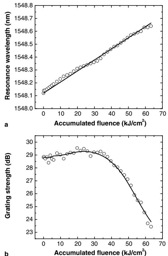
Fig. 2. Resonance wavelength: (a) and grating strength (b) of the FBG as a function of accumulated femtosecond laser fluence. The single pulse fluence was 124 mJ/cm<sup>2</sup>.
