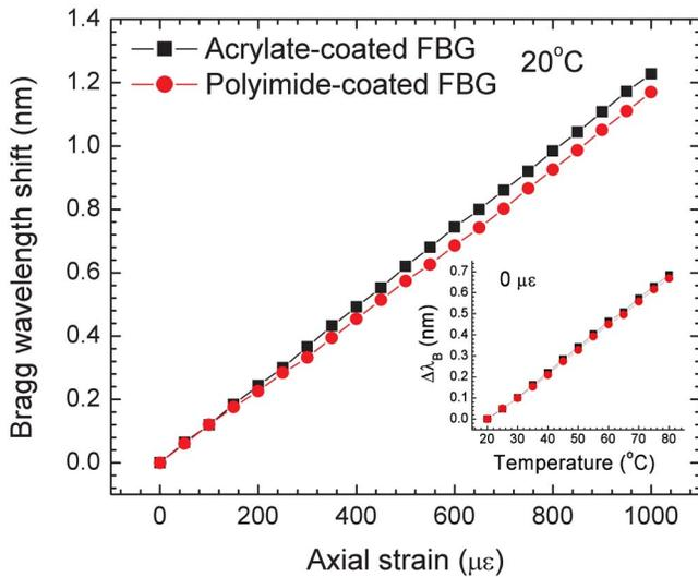
FIG. 3. (Color online) Dependences of the Bragg wavelength shifts of the acrylate- and polyimide-coated FBGs on the axial strain at 20 °C. The inset shows the temperature dependences of the Bragg wavelength shifts of these two FBGs without axial strain.
