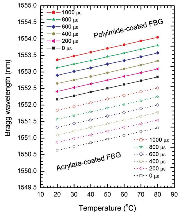
FIG. 2. (Color online) Bragg wavelengths of the acrylate- and polyimide-coated FBGs as functions of temperature under different axial strain values.
