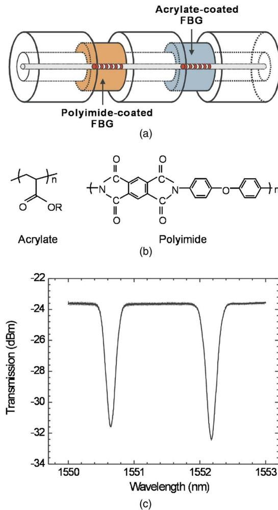
FIG. 1. (Color online) FBGs with different polymeric coatings: (a) illustration of the FBGs used in this study, (b) molecular structures of acrylate and polyimide, and (c) transmission spectrum of the FBG sample with acrylate and polyimide coatings.
