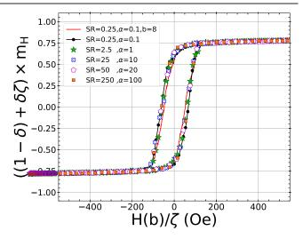
**Figure 4.** Invariance of MH loops. We combine RG scaling of magnetic quantities, larger time step with block size, and  $SR/\alpha$  scaling to predict the behaviour of prohibitively long fine-grain (b=1) simulations. b=4 unless otherwise noted.
